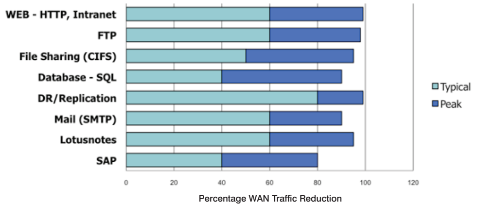
Figure 2 – Application response improvements achieved by reducing the amount of data on the WAN using compression, WAN memory and TCP acceleration.
